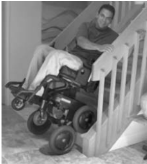
Photo 5: iBOT™ wheeled mobility system with stair climbing capability
